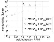
**Figure 1.** Dependence of conductivity on block composition and polyaniline content as measured by a four-point probe in ambient conditions from 1 cm  $\times$  1 cm films (30–50  $\mu$ m thick).
