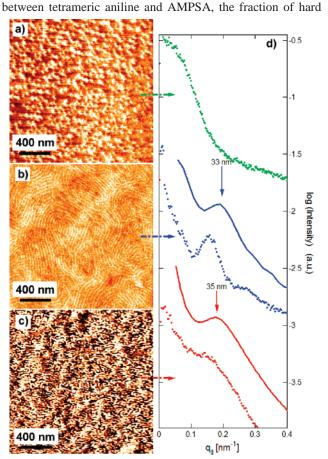
**Figure 2.** Left: phase contrast TMAFM images (a) (AMPSA)<sub>23</sub>-b-(MA)<sub>290</sub>, (b) 4EB<sub>11.5</sub>/(AMPSA)<sub>23</sub>-b-(MA)<sub>290</sub>, and (c) PANI(AMPSA)<sub>1)2.3</sub>/(AMPSA)<sub>23</sub>-b-(MA)<sub>290</sub>. Right: (d) azimuthally averaged SAXS scattering profiles (solid lines) with superimposed azimuthally averaged radial profiles of 2D Fourier transforms (dotted lines) from the AFM images on the left.
